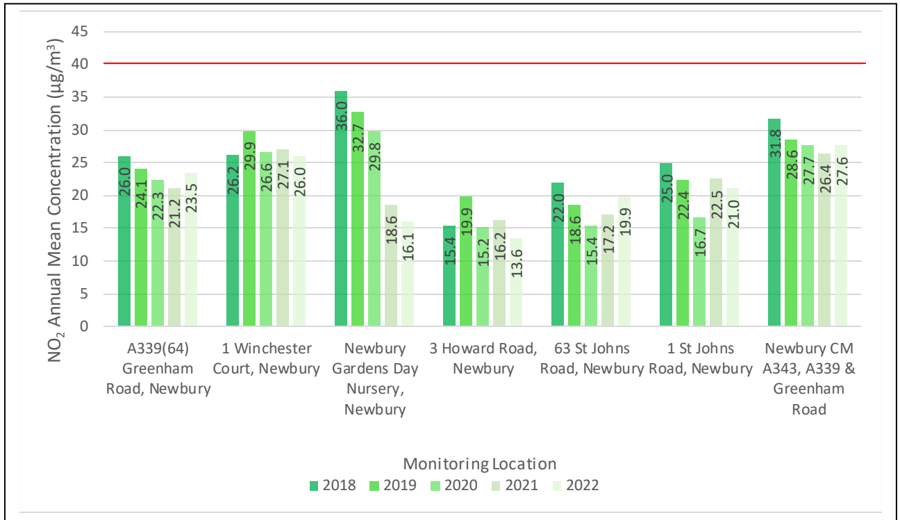
Figure 2: Diffusion tube Annual NO 2 concentrations at Newbury AQMA from 2018 to 2022
